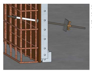
STEP THREE: SLIDE ASSEMBLED PLASTIC SLEEVE WITH CONES OVER THE TIE BAR.
