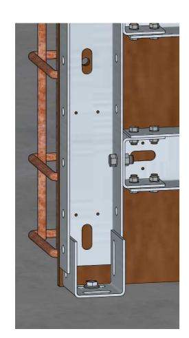
STEP ONE: PRE-DRILL HOLES FOR TIE BARS IN PLYWOOD.
