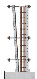
STEP FIVE: LOOSELY POSITION SECOND SIDE OF FORMWORK MAKING SURE ALL TIE BARS FIT THROUGH THE PRE-DRILLED TIE HOLES AND LOOSELY SECURE BY USING PLATE AND WING NUT.
