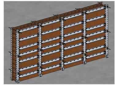
STEP SIX: TIGHTEN ALL THE WING NUTS UNTIL THE ASSEMBLED PLASTIC SLEEVE HAS BEEN FIRMLY SECURED AND THE DESIRED WALL THICKNESS HAS BEEN ACHIEVED.
