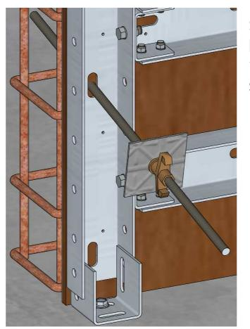
STEP TWO: POSITION TIE BAR THROUGH THE PLYWOOD HOLE. LOOSELY SECURE PLATE AND WING NUT.
