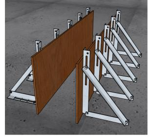
STEP SIX: FIT ALL PLY (FROM BEHIND) USING 20-25MM SCREWS. PLY TO BE A MIN. 18MM STRUCTURAL GRADE.
