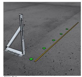
MARK THE LINE OF THE SHUTTER DEDUCTING THE PLY THICKNESS, THEN MARK POSITIONS OF RAWL BOLTS REQUIRED TO FIX DOWN THE BRACKETS. CENTRES OF THE
