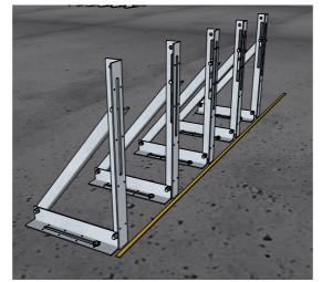
STEP THREE FIX DOWN ALL REQUIRED BRACKETS. FOR ALIGNING THE BRACKET SYSTEM PLUMB THE FIRST AND LAST BRACKET ONLY, LOOSEN THE BOLTS ON THE DIAGONAL MEMBERS OF THE REMAINING BRACKETS. ATTACH A STRING LINE TO THE TOP OF THE FIRST AND LAST BRACKET MAKING SURE IT IS TIGHT. ADJUST EACH BRACKET INDIVIDUALLY, BRINGING THE FACE OF THE UPRIGHT MEMBER TO THE STRING LINE BEFORE FULLY RE-TIGHTENING THE BOLTS WITH AN IMPACT WRENCH
