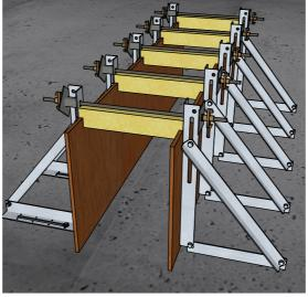
STEP SEVEN (OPTIONAL): SECURE OPPOSITE BRACKETS WITH TIE BARS IF TIE BARS ARE INCLUDED IN YOUR DESIGN. GENERALLY TIE BARS ARE NOT REQUIRED FOR THE FAST FORM BRACKET SYSTEM. IF BARS ARE USED A SPACER IS RECOMMENDED (AS SHOWN)
