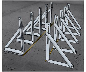
AFTER ALL THE BRACKETS ARE SECURED, YOU ARE READY TO FIX THE PLYWOOD TO THE BRACKETS WITH SCREWS.
