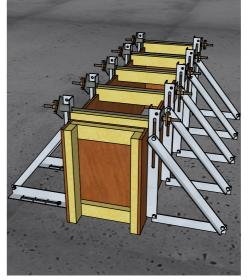
STEP EIGHT: FIT IN STOP-ENDS (SUPPLIED BY CLIENT) AND TIGHTEN ALL TIE BARS (IF REQUIRED). FIX ACCESS AND HANDRAILS IF REQUIRED (NOT
