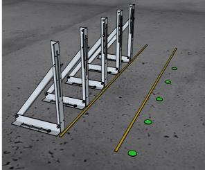
REPEAT PROCESS FOR OTHER SIDE OF THE BEAM. IF IT'S A SLAB SIMPLY CONTINUE THE PROCESS AROUND THE POUR. IF THE BRACKETS REQUIRE SECURING WITH TIE BARS, MAKE SURE THAT THE SLOTS IN THE VERTICAL MEMBERS OF OPPOSITE BRACKETS
