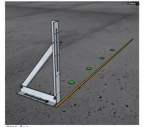
FIX DOWN THE FIRST BRACKET. REMEMBER TO POSITION THE CONCRETE BOLT AT THE BEGINNING OF THE SLOT IN THE HORIZONTAL MEMBER AS THIS WILL PREVENT THE BRACKET FROM BEING PUSHED AWAY FROM THE SHUTTER. FIX ALL RAWL BOLTS WITH A 110V IMPACT WRENCH. BRACKETS SIZE 150-800 REQUIRE ONE BOLT AND BRACKETS SIZE 1200-1800 REQUIRE TWO BOLTS.
