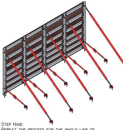
MOVED. THE SYSTEM DOES NOT HAVE TO BE REPEAT THE PROCESS FOR THE WHOLE LINE OF THE WALL. ONCE ALL THE PLYWOOD IF FIXED FORM SYSTEMS! A COMPETENT PERSON SHOULD LINE IN AND PLUMB UP THE WHOLE PANEL. EQUIPMENT SHOULD BE USED.
