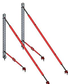
STEP TWO: REPEAT FOR THE NEXT UPRIGHT USING THE HORIZONTAL BRACE TO SET THE DISTANCE APART.
