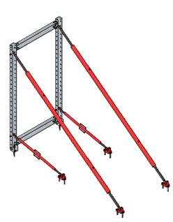
STEP THREE: LOOSELY BOLT BOTTOM AND TOP HORIZONTAL JOINING MEMBERS USING THE CORDLESS IMPACT WRENCH.
