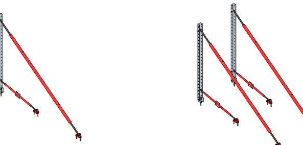
STEP ONE: DRILL AND FIX FIRST UPRIGHT TO THE LINE OF THE WALL MINUS THE PLYWOOD THICKNESS. FOLLOW BOLT MANUFACTURER TECHNICAL SPECIFICATIONS AND INSTALLATION GUIDES TO PROPERLY SECURE THE CONCRETE BOLTS. EACH PUSH/PULL PROP TO BE SECURED ON INDIVIDUAL FOOT. TWO CONCRETE BOLTS PER EACH INDIVIDUAL FOOT TO BE USED.
