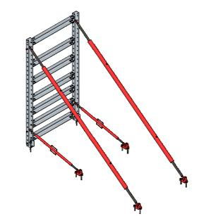
STEP FIVE: TIGHTEN ALL BOLTS AND PLUMB THE UPRIGHTS. PLUMB UP THE UPRIGHTS USING A SPIRIT LEVEL AND ALTERING BY TURNING THE PUSH-PULL PROP ONE WAY OR THE OTHER
