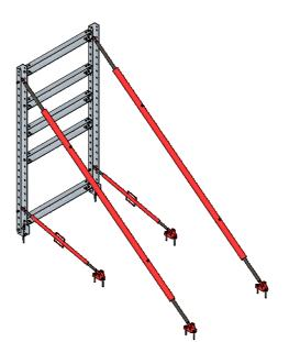
STEP FOUR: FILL IN REMAINING HORIZONTAL JOINING MEMBERS.
